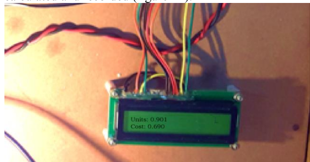
Fig. 14. E-Monitoring calculating the units of electricity consumed and cost accordingly
